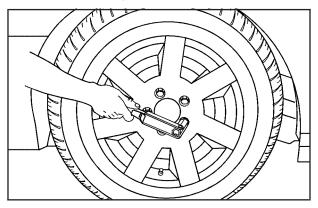
Loosen the wheel nuts, but do not remove them yet, using the wheel wrench. Turn the handle about 180 degrees, then return the handle back to the starting position. This avoids taking the wrench off the lug nut for each turn.
